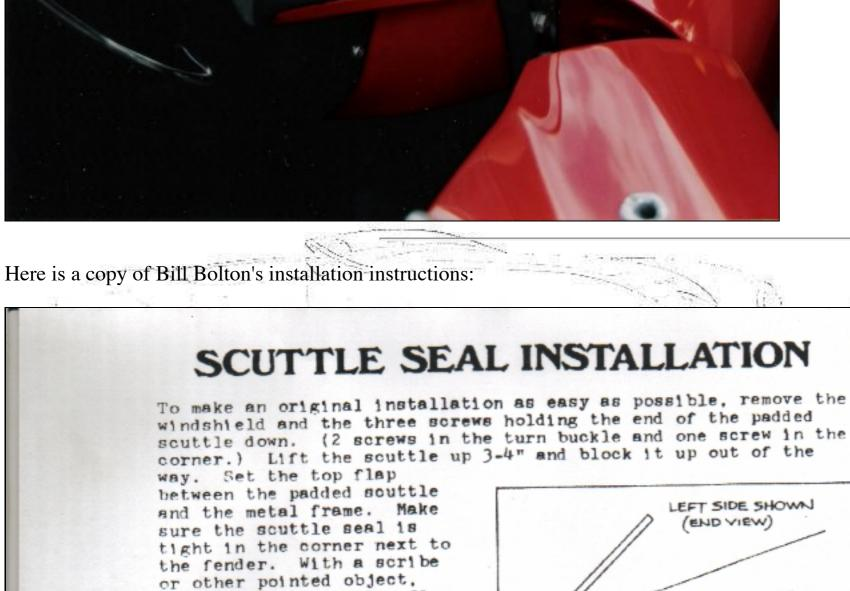
Cut the scuttle seal with a razor blade at cuts A & B back to the leading edge of the metal frame (the one the rivets went through) Then cut across the facing edge of the metal frame. Cut the lower end of the scuttle just above the door
