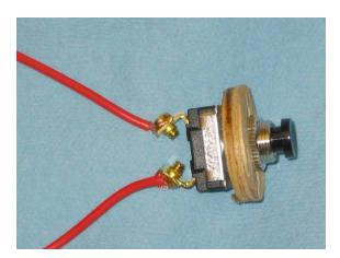
Power comes from a switched terminal on the ignition switch, and is connected to the new red wiring through an in-line fuse holder. From the other side of the switch, a new red wire carries power to the pump. The "negative" side – black wire - of the pump is grounded at the mounting bracket.
