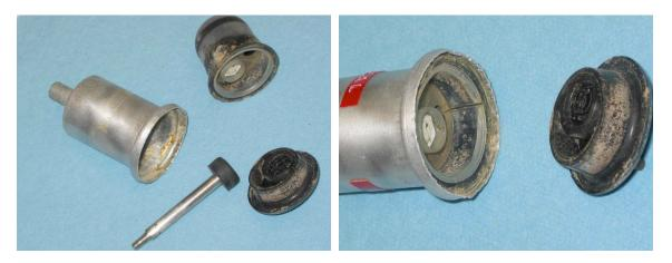
To provide enough depth for the switch in the canister I cut a slot in the plastic face plate. The slot also provided space for the switch wires to exit the canister.
