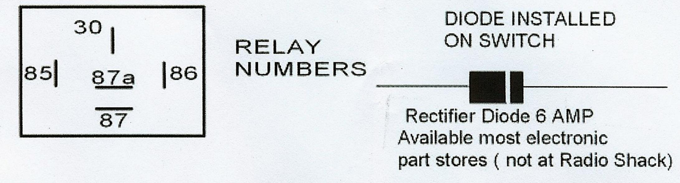
NOTE: If the diode is not used only the headlights will come on when the wipers are running. With the diode connected the parking and tail lights will also be on. Normal function of the lighting will remain as stock.
