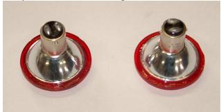
The rubber then needs to have a hole bored through the center of it so that the bulb can go through. I found that a 1" diameter hole is best to allow the cone shape of the bulb to fit. Rubber is a difficult medium to bore a 1" hole in. I tried a spade type wood drill, which doesn't work the best. Then I got a 1" hole saw that did a fairly good job.
