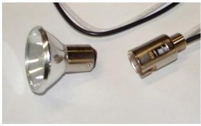
As it turns out the bayonet mount bulb and socket are much more substantial than the pin mount. The reflector is made of aluminum rather than glass and has a plastic cover over it to protect the actual bulb, kind of like a miniature sealed beam unit.
