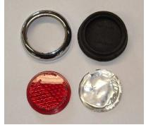
The original reflector for my car, a BT7, is not flat, but has a well in the back that the MR11 fits down into. I've found that Longbridge 100-6s and the Moss aftermarket reflectors do not have this well.
