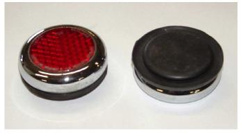
Then you need to take it apart by gently prying the rubber out of the chrome ring with a small screwdriver. Be careful not to stick the screwdriver in too far as you could break or chip the plastic lens. If an original Lucas reflector unit, it should have a heavy aluminum foil backing on the lens, which needs to be removed by getting under its edge and pulling it free. Here is what you will have when you get everything apart:
