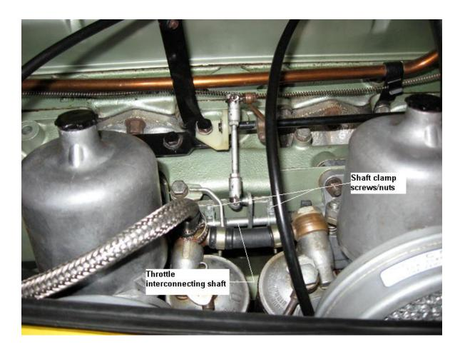
5. Rotate each throttle plate fully closed by turning its shaft as far as possible (counterclockwise, as viewing the end of the shaft from the front of the car). Each shaft can be rotated and held in the throttle-closed position using the shaft lever (to which is attached the carb return spring). With each throttle plate held fully closed, re-tighten its shaft clamp screw/nut.
