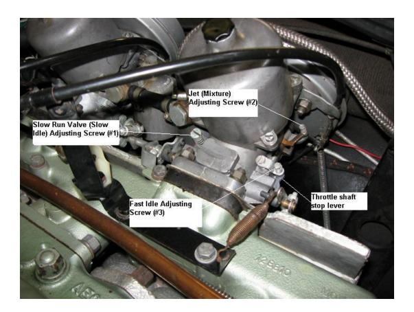
4. There is an interconnecting shaft between the carburetors that makes both throttle plates open and close together. Loosen the screws/nuts (5/16") on the interconnecting shaft clamps so that each throttle plate can be rotated independently of the other.
