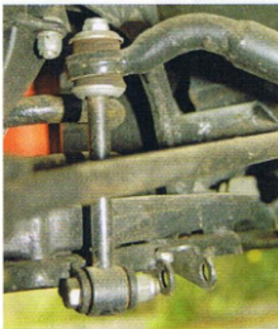
See how the anti-roll bar is extended to connect further out on the lower wishbone. The original bracket is left in place, showing us where the original link attached
