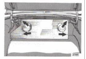
Fig. 23. The evaporator cover mounting points.
