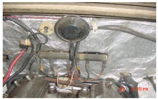
A 420 resistor set-up
