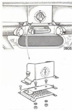
Fig. 21. Attachment of control unit panel.
