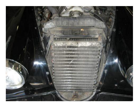
The main condenser mounted in front of the radiator.
