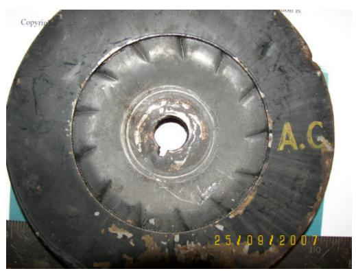
An E-type air conditioning Alternator Fan - the "A.C." designates this as a reverse unit for use only when air conditioning is fitted
