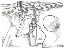
Fig. 22. The receiver/drier mounting.
