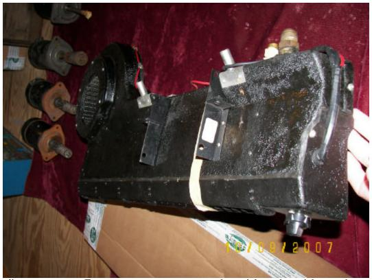
Radio mounts on an E-type evaporator case – note the serial number sticker on the near bracket
