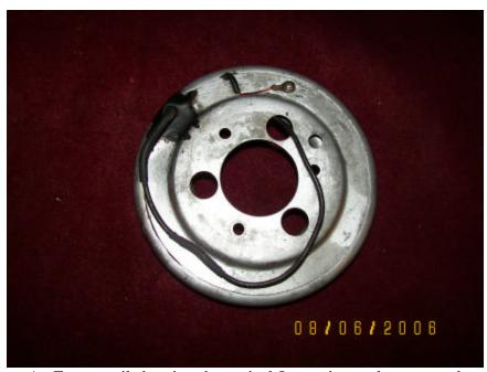
An E-type coil showing the typical Jaguar internal mount and finish
