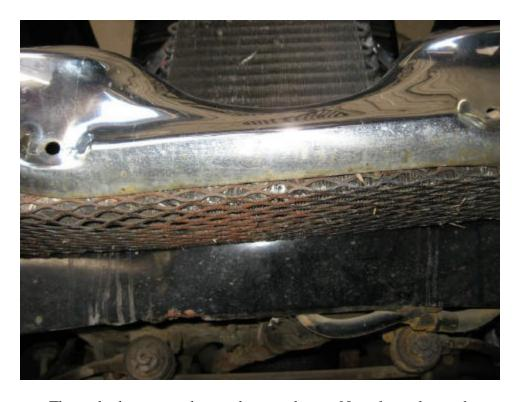
The under bumper and secondary condenser. Note the rock guard.
