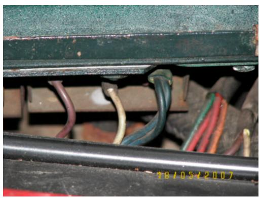
A MK 10 / 420 G resistor under the right fender
