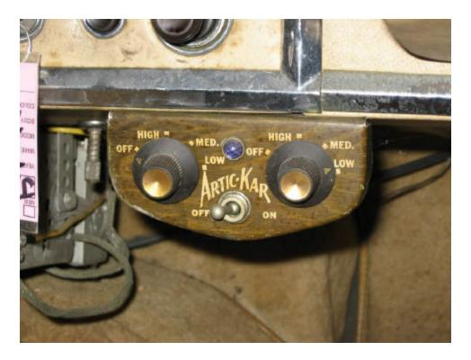
A typical set of control switches. There are two fan speed switches and a compressor on off switch with a blue ON lamp. Note the period LOGO and the wood grain lithograph is unique to this author.
