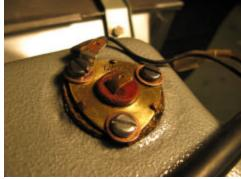
Otter<sup>®</sup> switch mounted in the header tank of a Series 1 E-type – Photo by Bill Beatty
