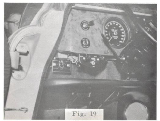
A period photo of a dual switch and temperature control installed in an S-type
