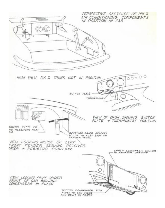
The drawings above and on the previous 2 pages clearly represent a 3.8 litre version – note the stylized brake booster to the left of the resistor above, and the "fixed" cool air vent on page 13. Also note that the controls are carried over from previous models and not centrally located as in later versions.
