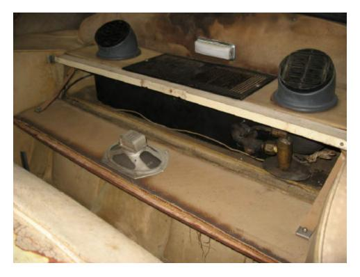
A more complete picture noting the rear compartment has been modified for the AC yet has been covered with the proper materials. This was typical in the period.
