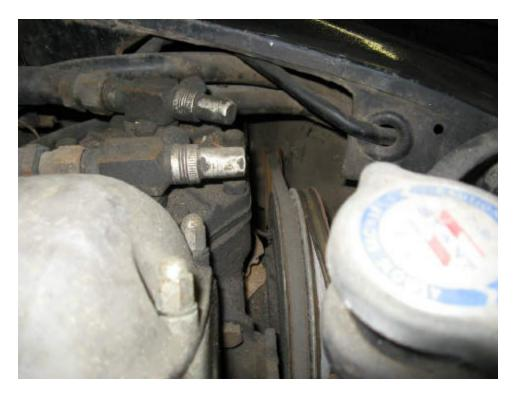
Of interest in this picture the inner wing has been cut to allow for the compressor. A box cover was fabricated for the wheel side to cover the opening and protect the compressor and generator (under the compressor).
