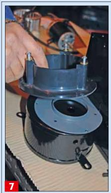
Offer up the motor plinth base and plinth before screwing to the heater body with the self-tap screws provided. Then the motor can be fitted, again with the screws provided (below)
