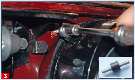
Fitting is the usual reversal of the removal process, making sure that any hoses are replaced and the supply pipes are carefully examined. This is being fitted with a rubber buffer under a bolt. Should the original bobbin type be required (see inset) they are available from SNG Barratt as part number C24792
