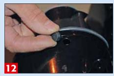
Fit the grommet into the hole used to access the grub screw
