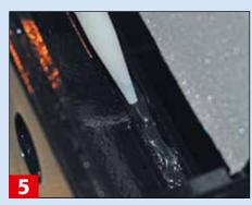
Silicon sealer is used around the inner flap aperture and the flap pushed close to make a permanent seal
