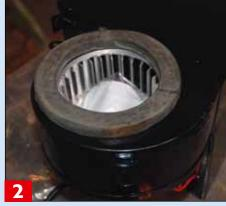
This seal from the fan to bulkhead was in good condition and could be reused
