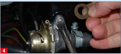
A replacement water valve has been fitted, again available new. The old seal can usually be reused as long as it is thoroughly cleaned
