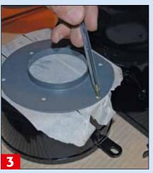
Clayton had the heater box stove enamelled (rather than powder coating due to the heat developed) before the next stage. Masking tape is applied to the heater box surface and the new heater plinth base is offered up to the heater body with the flat end close to the box and the initial curve of the plinth following the contour of the heater box fan area. Make a mark through the holes for later drilling. Offer up the resistor anywhere alongside the plinth and mark the holes
