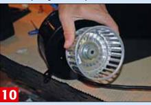
Offer the new fan over the motor spindle noting that the shaft is a D-shape with a suitable D-shape hole in the fan centre
