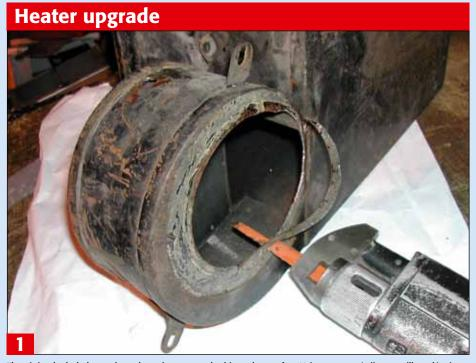
The air intake hole has to be enlarged to accept the bigger heater fan. Using a cutter (a jigsaw will work) trim away excess metal so that the hole meets the required 120mm. Try to keep parallel to the original hole edges
