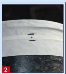
Measure down 20mm from the top of the heater box fan area and scribe a line. Then measure a further 10mm from that line and make another mark. Make a central mark (5mm down from the first) and then drill a pilot hole with a small drill bit. Follow this with a 10mm drill bit. The hole is to allow access for an Allen key later used to secure the new fan
