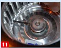
Arrange the fan so that it is close to the heater body but with enough clearance to miss while spinning and then secure with the grub screw using a long Allen key
