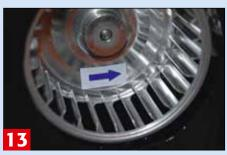
Couple the wires up to the battery and make sure that the rotor fan spins the right way (note the arrow). Swap the wires around if not. As the motor is isolated from earth it is not polarity dependant
