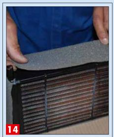
Apply foam to the outside of the heater matrix. This is to cushion the matrix against the heater body. Then lower the matrix into the heater body with the outlet pipes uppermost (see below)
