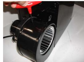
8. Insert rubber blanking grommet into 10mm hole.
