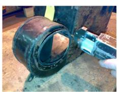
3. Drill a 10mm hole, 20mm down from the motor mounting surface on the fan wheel scroll.
