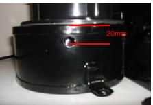
4. Using motor mounting plate as a template, drill three 2.7mm holes for securing the new motor mounting plate. (Ensure the motor mounting plate is centrally positioned about the spindle hole before drilling).
