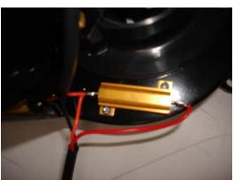
13. Use 12v power supply to ensure motor is rotating in anti-clockwise direction when looking at fan wheel.
