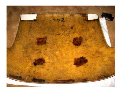
Glued carpet felt to four locations on the underside of the hardtop shell. This buffers the headliner metal frame from the fiberglass shell.
