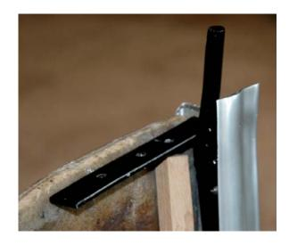
Applied 3M caulk to the channels in the bottom cant rail and positioned the rail on the top shell. This job requires two people! After properly aligning the rail, six stainless truss head screws can be screwed into place through the side and bottom cant rails into the steel spigot pin.
