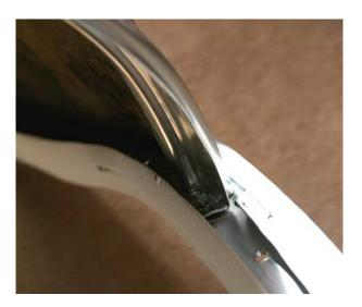
I had saved the five small original rubber seal pieces that were used as spacers/cushions between the headliner and the upper backlight aluminum trim. These were glued in place at the same locations on the inside of the top shell.
