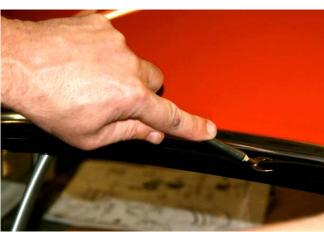
After installing the locking strips and cleaning up the silicone spray residue, the backlight installation was complete. Now, it is back home to put the seals on the bottom cant rail.
