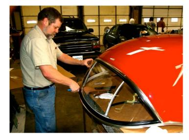
These are a few images of the locking strip being "run in" to the larger seal. As always, the right tool for the job is key. John's assistant trimmed the locking strip to the proper length.
