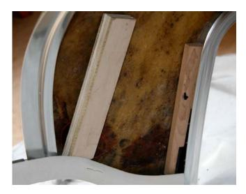
I then used a block of wood on each side of the top to spread the top toward the outside of the bottom cant rail and inserted two #10 stainless truss head machine screws with washers and nuts to link the bottom cant rail to the backlight top aluminum trim. After tightening the fasteners the wood spacer blocks were removed.
