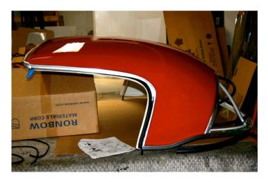
To get a feel for how the top and bottom seals would ultimately join together the installer slid the pieces together on the rails. The upper backlight glazing rubber was part number 27H9594. The lower glazing seal was part number 27H9595.
