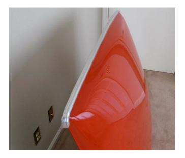
Applied 3M caulk to the channels of the side cant rails and pushed the rails onto the top shell. Temporarily screwing in the corner braces and the small aluminum plates helped pull the side rails into place.
