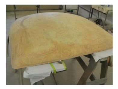
The fiberglass shell is very flimsy without the supporting aluminum hardware that serves as an external skeleton for the top. It had developed some cracks and blemishes over the years.
