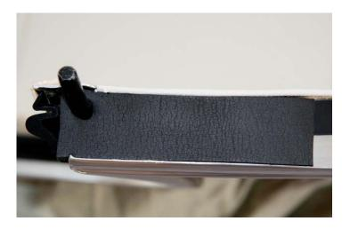
The narrow (3/4") packing strip for the bottom cant rail (27H9686), was then glued into place. The piece in the image below was cut off to butt against the spigot pin pad.
