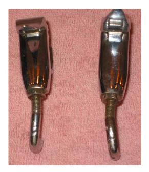
The rear mounting hook/plate/wing nut assembly was also in good shape but I did decide to replace the hooks and again sourced them from Cape International. I ordered new mounting plates, but like the shape of the originals so I will stick with them.
