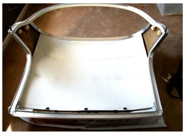
The aluminum backlight braces were then installed. I stuck 3M body caulk under the heads of the two chrome machine screws that went through the backlight upper aluminum trim and into the braces to help seal out water.
