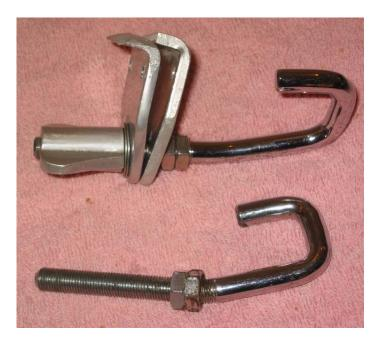
The steel locating spigots just needed some cleaning up and painting. They were painted black and new truss head stainless screws were purchased for assembly
