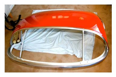
I was then able to flip the top over and install the front pad. The screws that fasten the front side braces needed to be withdrawn so that the triangular clip on the side of the front pad could be pushed into place between the two screw locations. The screws were then replaced. The front rail header seal, part number 27H9597, was then cut to fit and glued onto the rear edge of the front aluminum rail.
