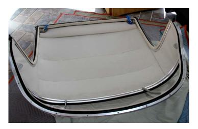
The wide (1 1/8") packing strip, to the left in the image at right, was glued over the narrow packing strip and it also was run to the back of the spigot pin pad. Then the header rail seal (27H9597) was lightly glued over the edge of the bottom rail and the windlace was pressed over it and the rail to give a finished appearance.
