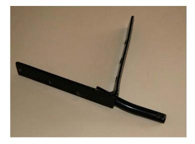
The headliner was torn and dirty and needed to be replaced. The headliner frame needed attention, too. It was a little rusty and the felt was in bad shape. The frame was painted black and new felt was glued in place.
