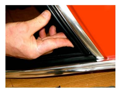
The installer used a silicon spray to temporarily soften and lubricate the rubber to make it easier to fit the plexiglass and the locking seal. Unfortunately, we discovered that my glass was not shaped properly.
