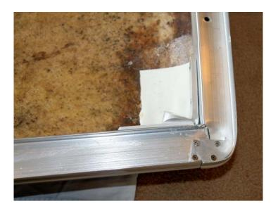
The original wood braces that mount on the side cant rails were rotten. I had new braces made to original specifications. These were screwed to the side rails with two truss head stainless screws.
