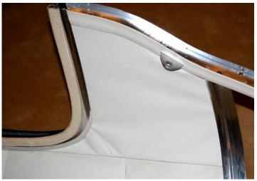
The hold down brackets that, along with large "J" hooks, clamp the hardtop to the cockpit were then inserted through the slots in the bottom cant rail and secured with two #10 truss head machine screws. I used the original quarter panel boards and recovered them with the headliner material. They were pushed into place and wrinkles were "massaged" out as much as possible.
