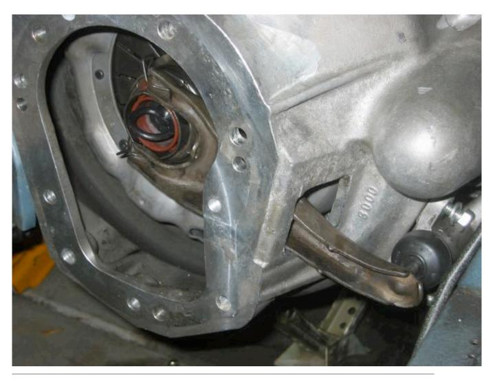
Here is a close up of the problem. This makes the bellhousing act as the fulcrum, which makes the clutch hard to operate and the slave rod to over extend.
