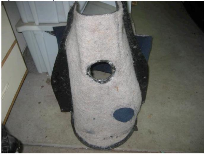
I then had my buddy weld some nuts to the back of an old MGB shifter boot beauty ring. I drilled four holes in the beauty ring and rivited it to the inside of the tunnel. Presto, captured nuts for the final beauty ring. (Note: these captured nuts have nothing to do with the Tranny/Motor mating ritual, don't get confused on me here)
