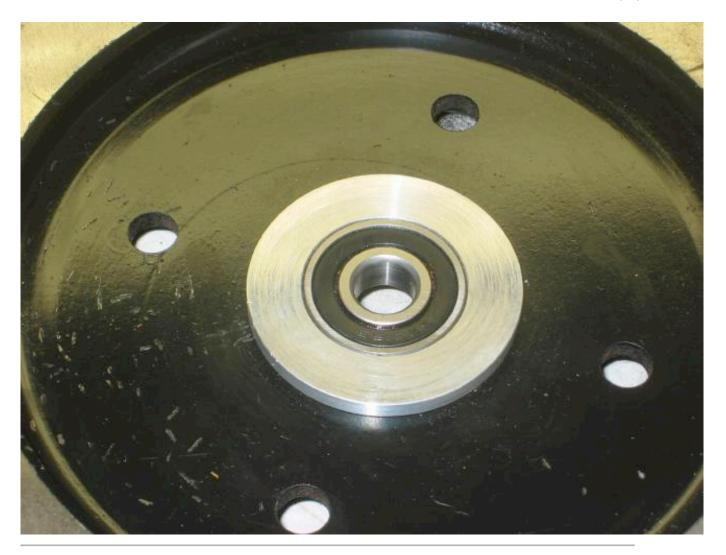
The failed brass style pilot bush. This was the brass pilot bushing supplied by Smitty with this kit. I tried it (actually two of them) but kept spinning them out of the flywheel. What a wild squeal this makes at take off. Very disconcerting. The aluminium one with the pressed in bearing looks more promising.
