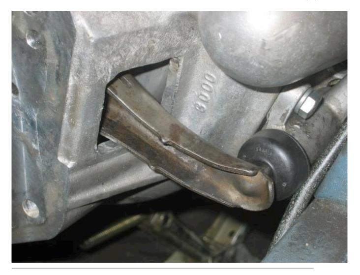
And a closeup showing proper clearance and sane slave pushrod length and throw.
