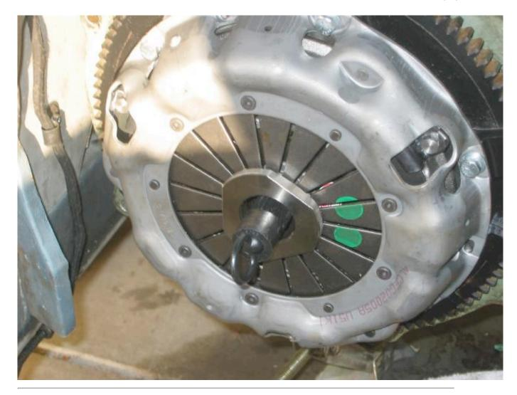
Now it is time for the test fit. Good thing I did this or I would have had to pull the transmission. Note that the clutch fork touches the bellhousing. There is not enough clearance with the BJ8 diaphram clutch. There was with the old spring type clutch.
