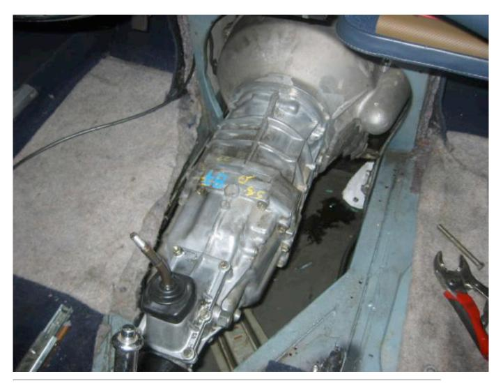
After the transmission is mounted up front I jacked up the rear of the transmission to get enough clearance to install the rear mounting adapter supplied by Smitty. Be careful as you do this as your throttle linkage will bind. You may want to remove the front linkage mount or at least keep an eye on this as you jack to keep from straining it.
