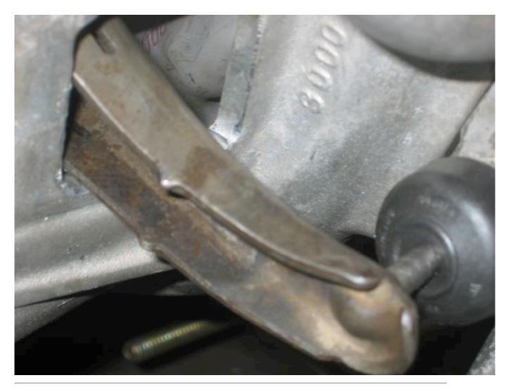
Here is how I solved the problem. The fulcrum pin is too short so I fabricated a longer one using a metric bolt cut to length, rounded the head and threaded to depth.
