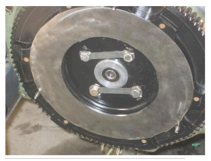
Pressure plate installed using the Smitty supplied clutch disk (thicker than stock Toyota) centered using a alignment tool (supplied in kit but available from Toyota)
