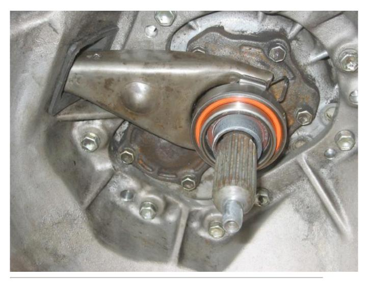
The entire thing then bolts right up to the motor. Alignment is key here. Do not allow the transmission to sag on the clutch and pilot bearing. I recommend using a tranny jack and a buddy although I do these alone with a roller floor jack so I know it can be done. Be careful I use some long bolts (5 inch) to guide the mating ritual of motor and tranny. Slow and steady here. It is one of the few times you will hear classical music coming from my garage.
