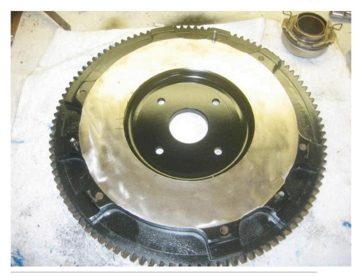
The Aluminium pilot bushing with bearing pressed in. This is supplied by Pete Delaney and is pressed in the flywheel. I "pressed" it in with a hammer and soft drift with a rubberized hunk of gasket to keep from buggering up the aluninium.
