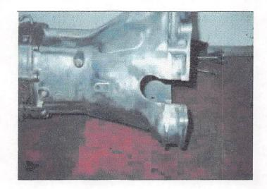
Looking at the front surface of the bellhousing, measure downward along the flange 4-1/8" from the bottom edge of the 1" hole in the flange and mark this spot. From this mark, measure straight back onto the side of the transmission 3" and make a second mark.
